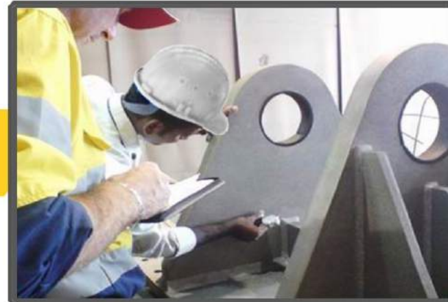
Blasting Surface Finish Check
