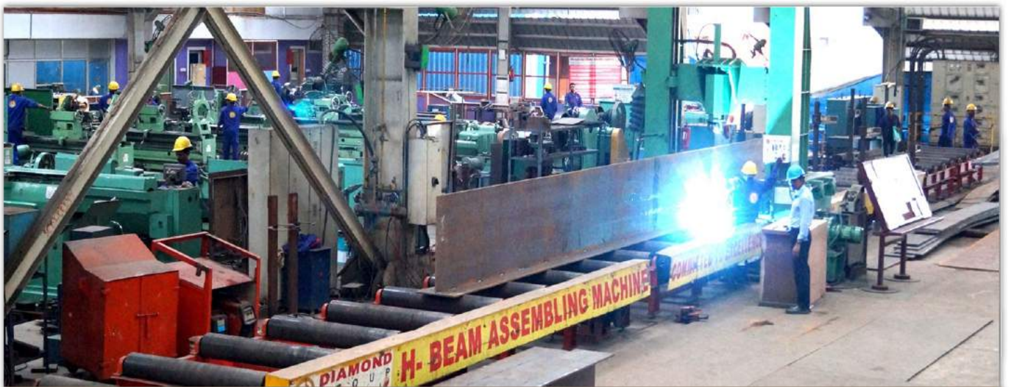
H-Beam Fitup Machine
